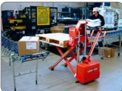
The height of the photocell can be adjusted. Highlifters: between 490 - 970 mm. Logiflex: between 550 - 920 mm.
