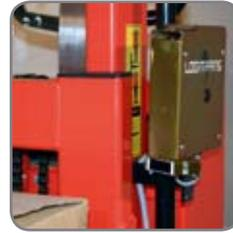
By means of the electric sensor, the forks raise when unloading material and lower when loading material.
