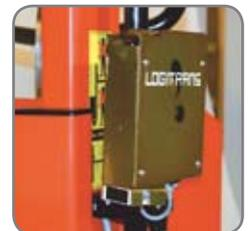
Control box has adjustable reaction time: from 1-10 sec.
