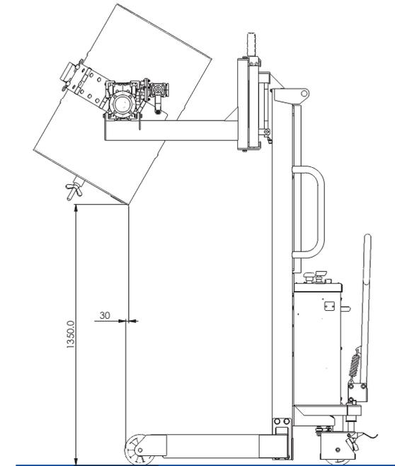
NOTE: STANDARD 205L STEEL DRUM USED FOR TIPPING DIMENSIONS. TIPPING HEIGHT WILL VARY FOR OTHER SIZED DRUMS
