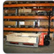
The Basic pallet truck shown being used in the component industry moving heavy goods.
