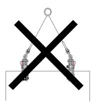
• Function lifting of loads in an horizontal position using 2 clamps at least and a lifting beam: the working load limit of each clamp is divided by 2.
