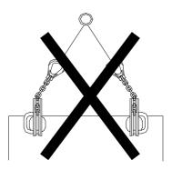
• Function lifting of loads in an horizontal position using 2 clamps at least and a lifting beam: the working load limit of each clamp is divided by 2.
