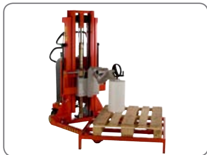
The pallet rack makes it possible to reach the reels from a various number of sides.
