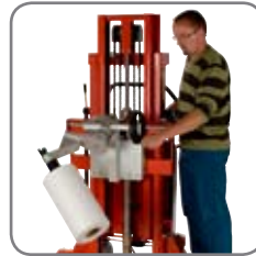
Rotation is performed manually, with or without gearbox.
