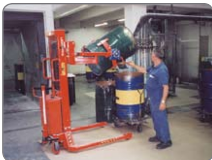
Manual drum turner is available for all Logiflex models. Electric drum turner is only available for the electric models.
